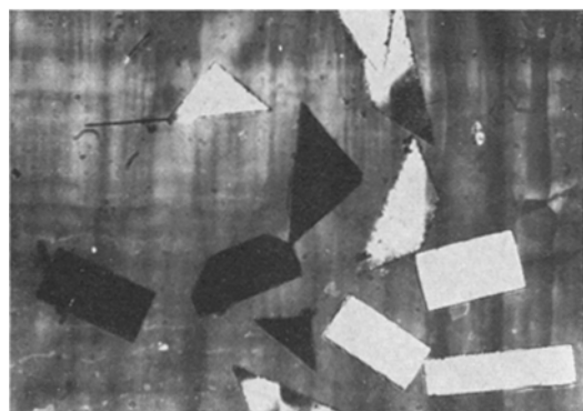
Figure 2 Nickel crystal platelets formed by reduction of \text{NiBr}_2 ( \times 10 )
